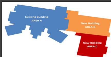
Building footprint divided into phasing areas. Area A consists of the existing building to be renovated upon completion of the addition.
