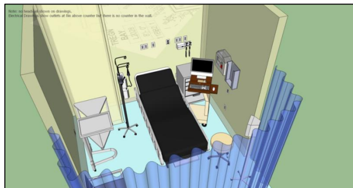
Figure 49 - Mock-up of a patient room for Tyson's Corner. A mistake found here was that electrical drawings specified outlets were to be placed 8" above the counter, but no counter exists in this room. Image courtesy of Shane Goodman.
