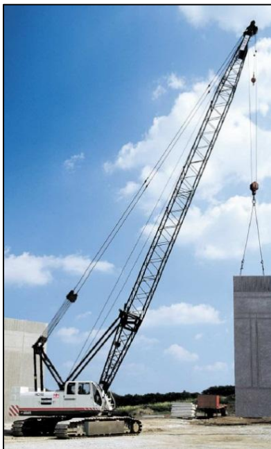
Figure 42 - 110-ton crawler crane selected for precast panel erection. Image from Carde Specific.
